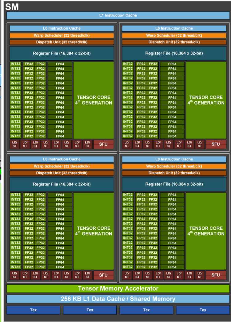
Nvidia GH100 SM architecture
