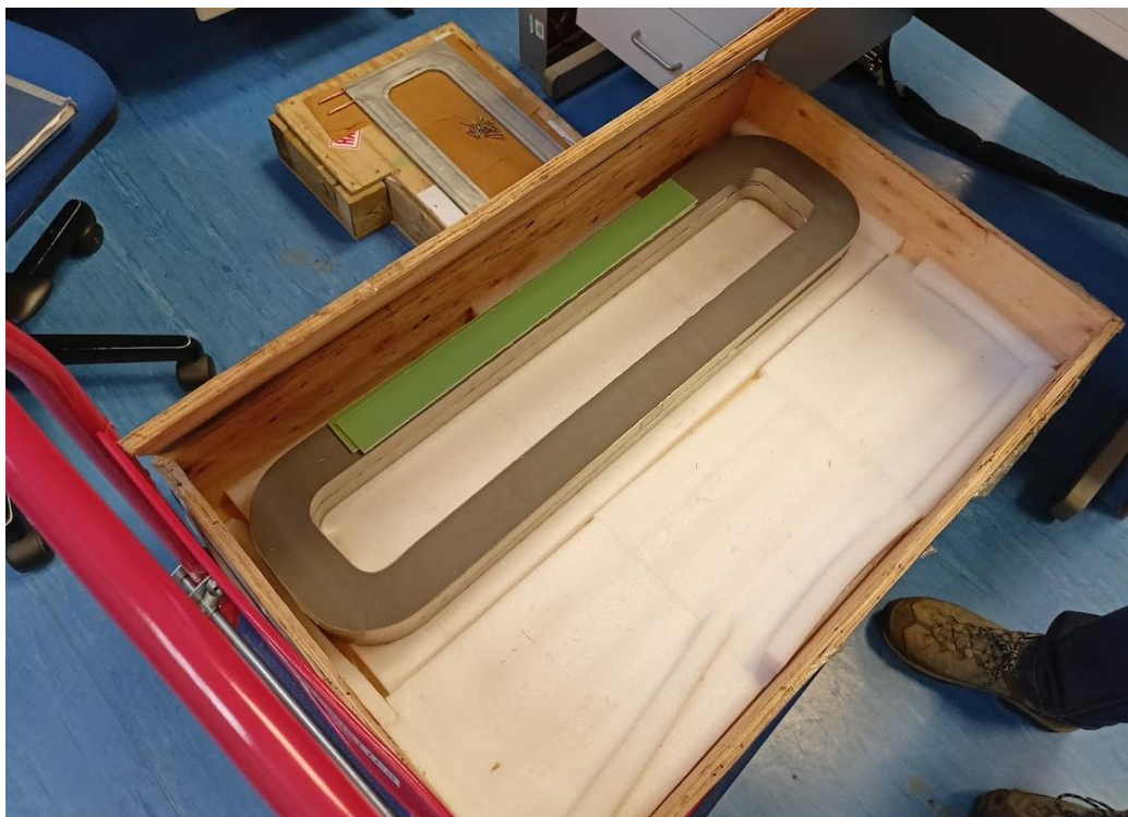
Figure 4: A prototype core to be tested for the FETS FFA RF cavity
