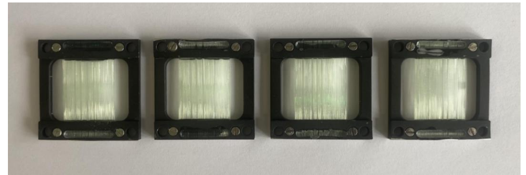
Figure 18: Scintillating fibre plane detectors built in the lab.
