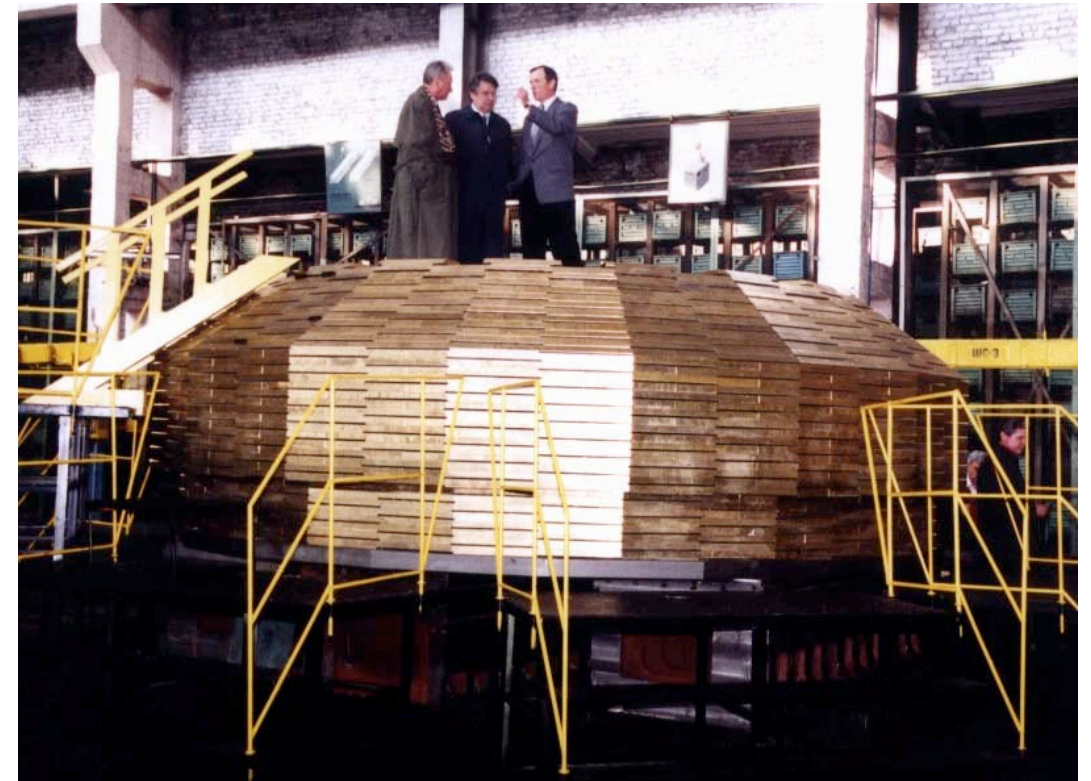
Completed HE brass structure
