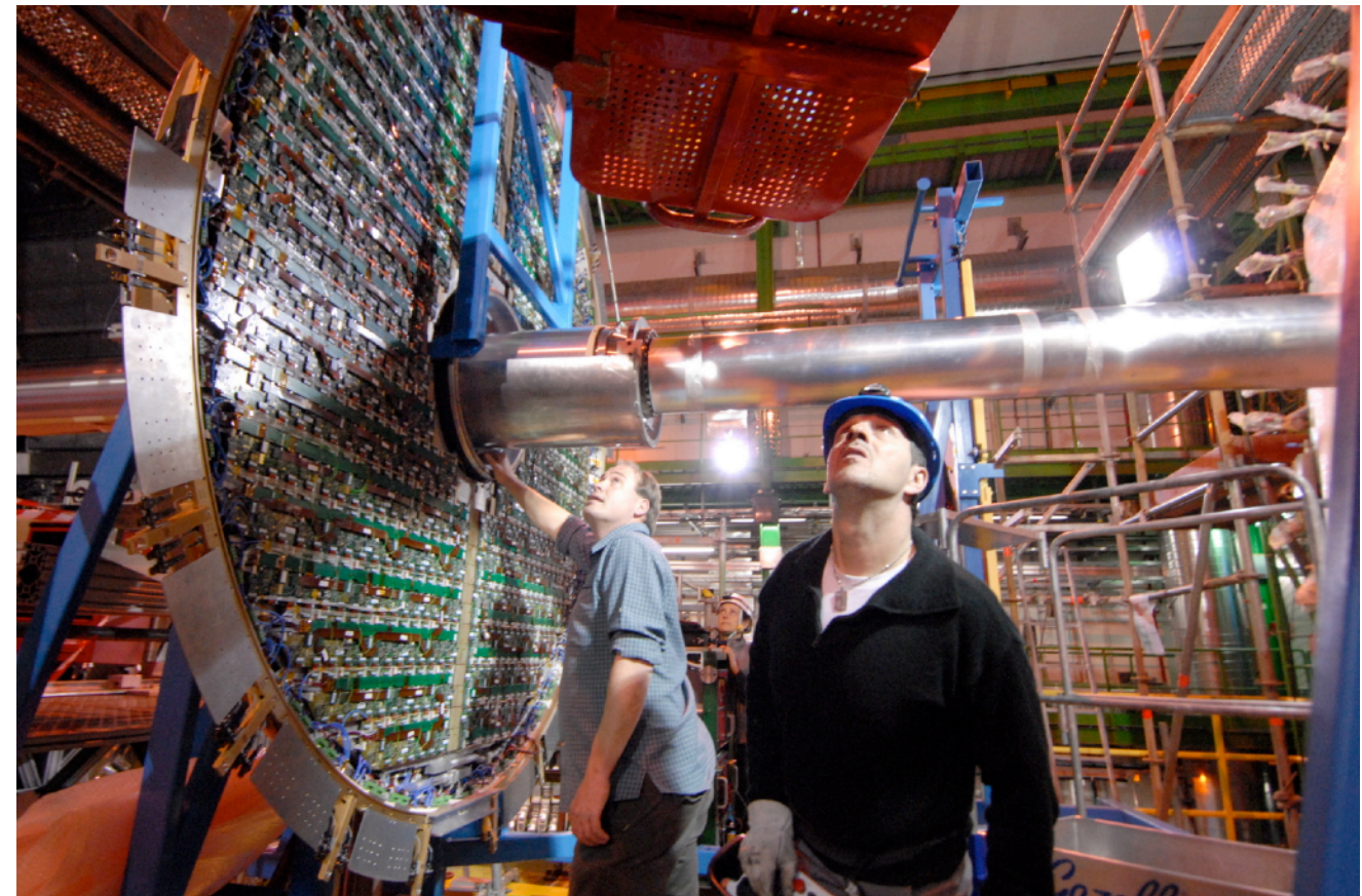
Preshower Dees positioned around beam pipe
