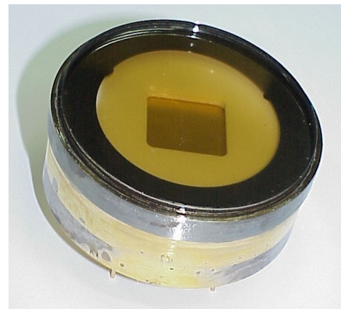
GEM with semi-transparent Photocathode (K-Cs-Sb)
