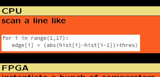
instantiate a bunch of comparators, get result in O(1) clock cycle
