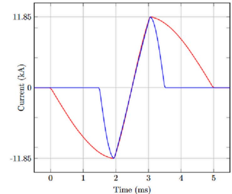
Changes in ramp shape requiring more RF cavities
