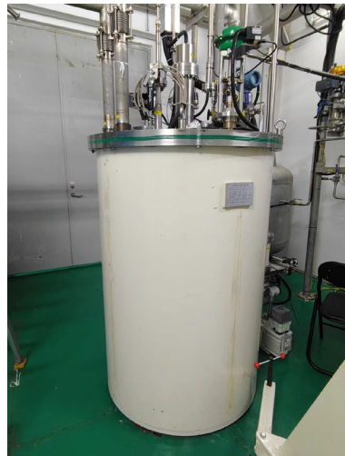
Hydrogen Loop(1.5 MPa@18~21K)
