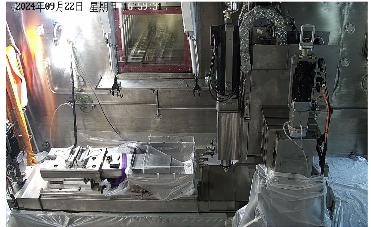
three-axis milling machine in hot cell
