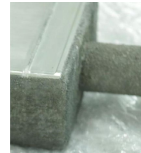
Electroplated cadmium layer of DWM 22
