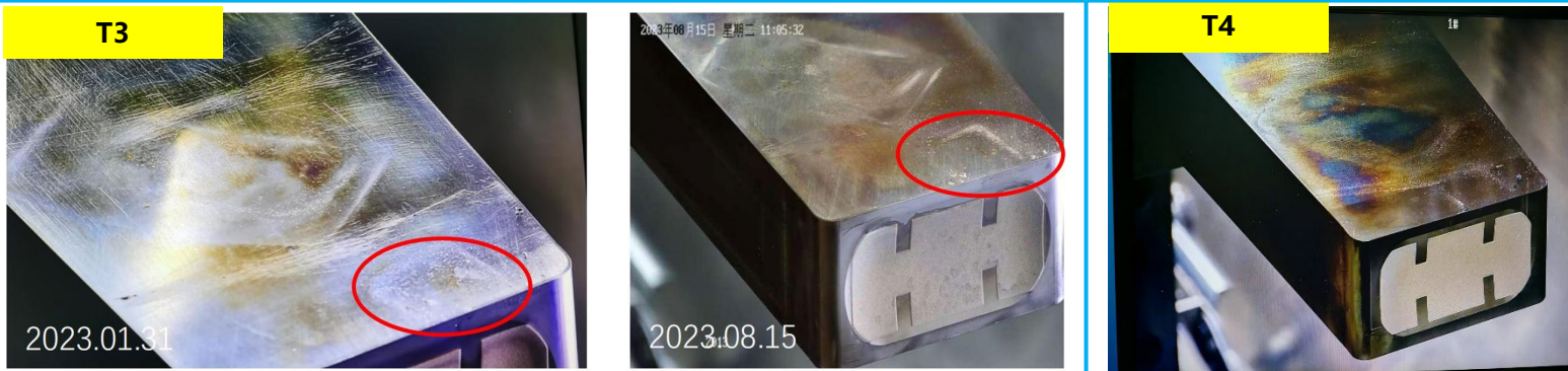
The decoupled cadmium layer powder on the surface of the target
