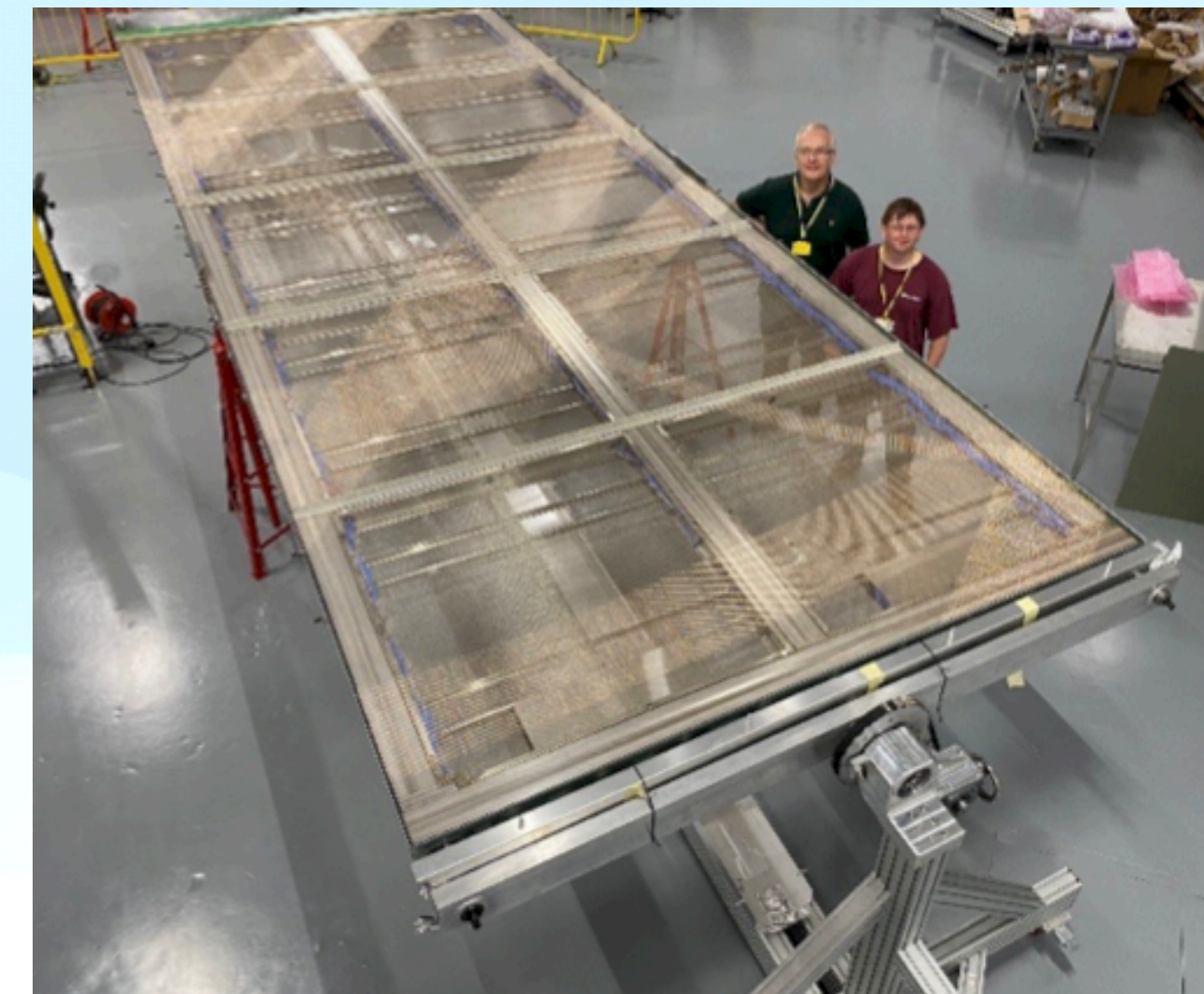
DUNE APA plane tested at Daresbury Lab
