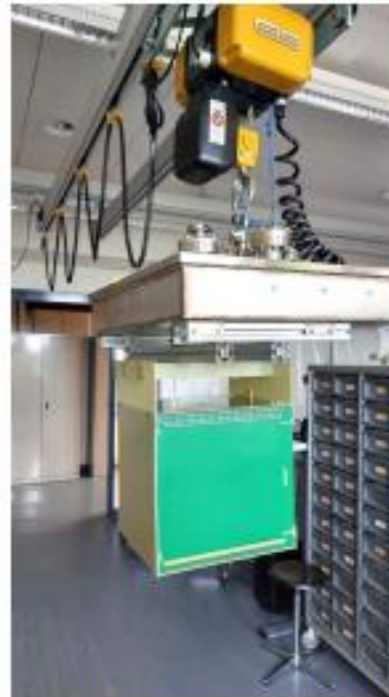
The cube TPC assembled and hanging on the top flange
