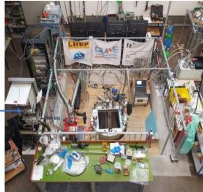
The laboratory at University of Bern with the LAr cryostat
