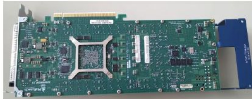
PCIe 16x board, 1 Intel Stratix 10 FPGA, 16 optical links
