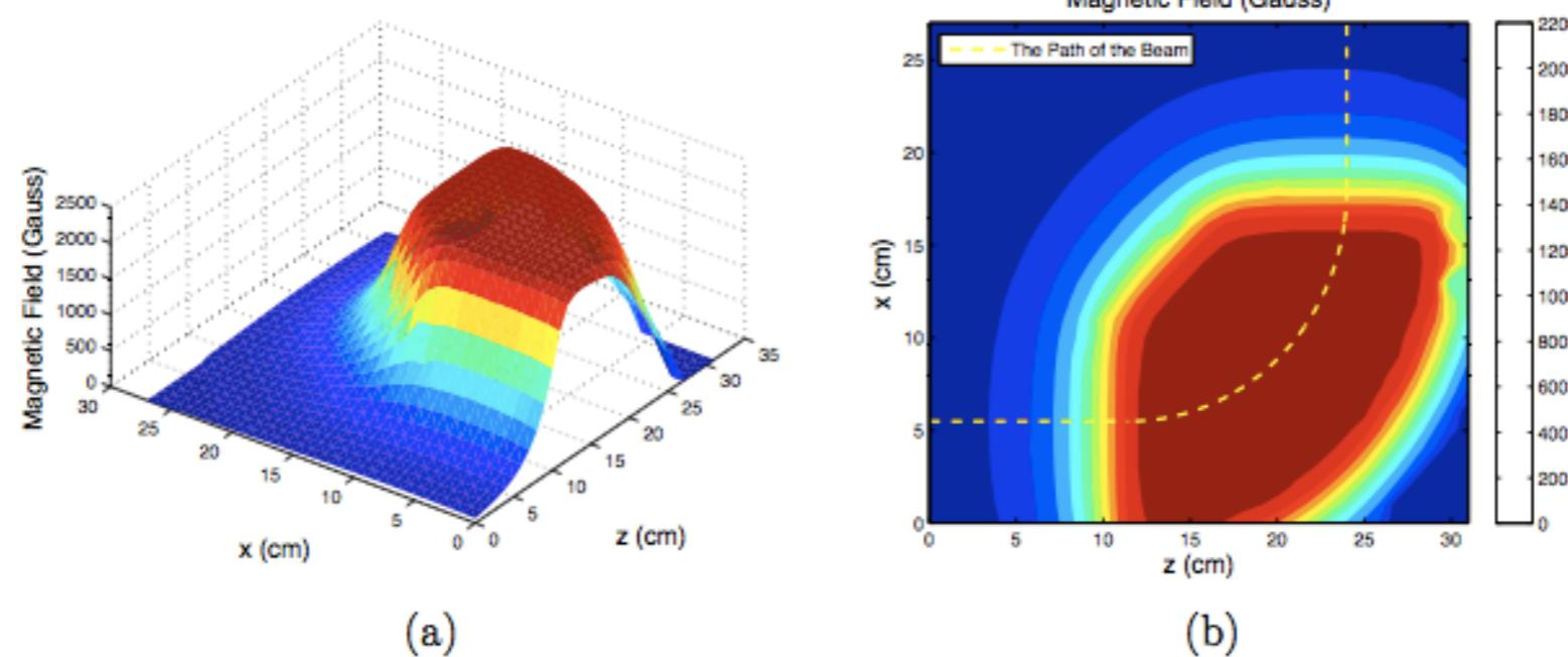
Magnetic field map of a dipole magnet.
