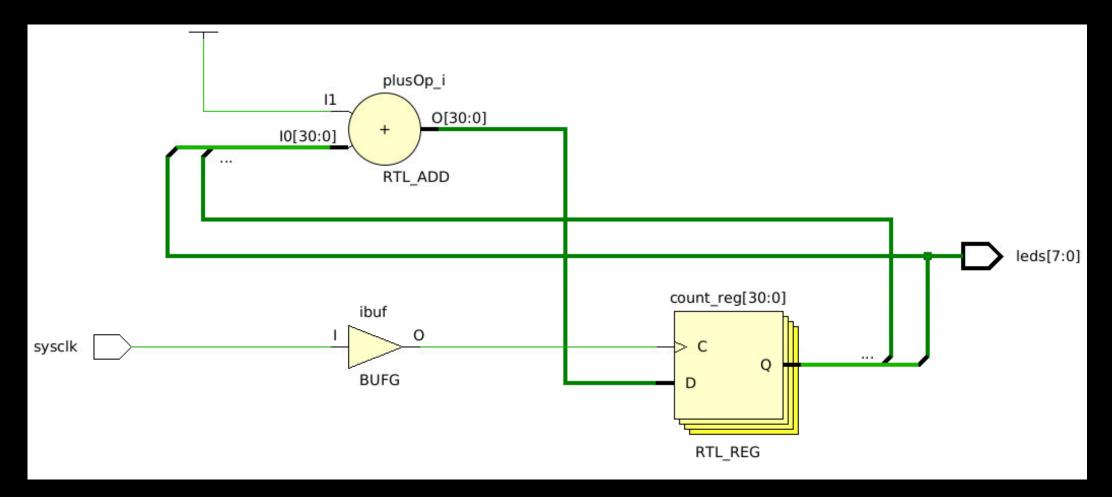
We won't use schematics today, but we will implement <u>this</u> design. Note inputs, outputs, blocks, signals, busses, constants, and a loop! Relatively easy to understand, but not very practical for complex tasks.
