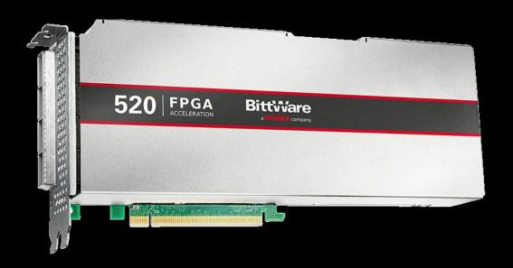
FPGA accelerator card based on Altera device
