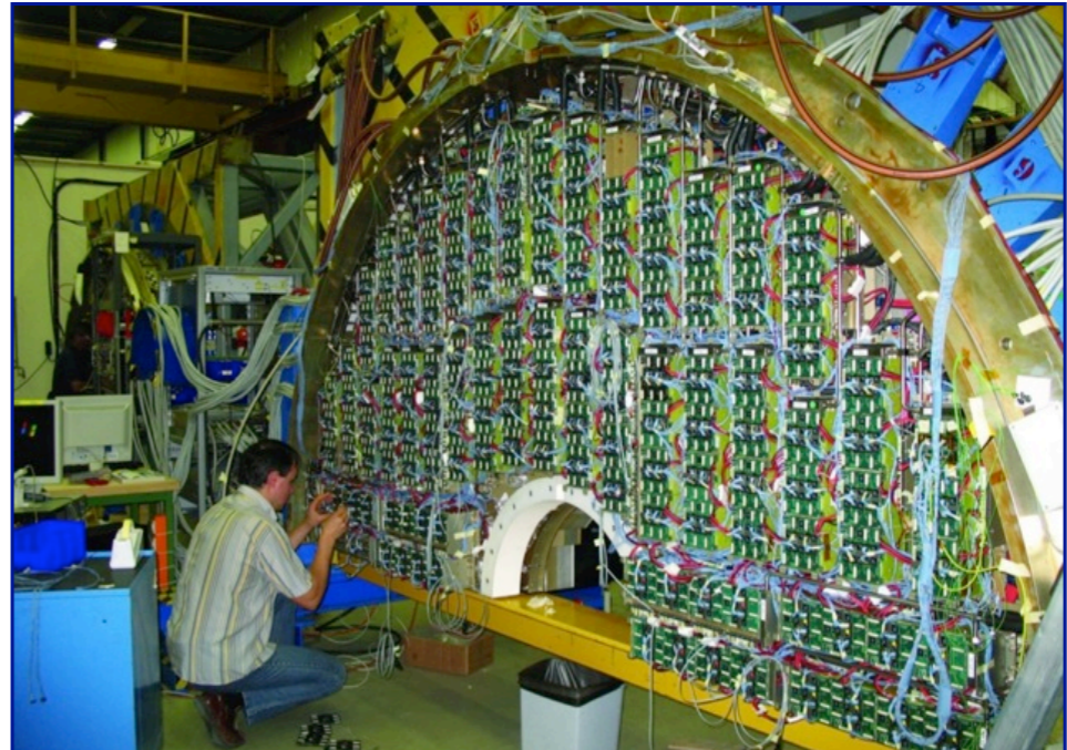
Installation of readout electronics
