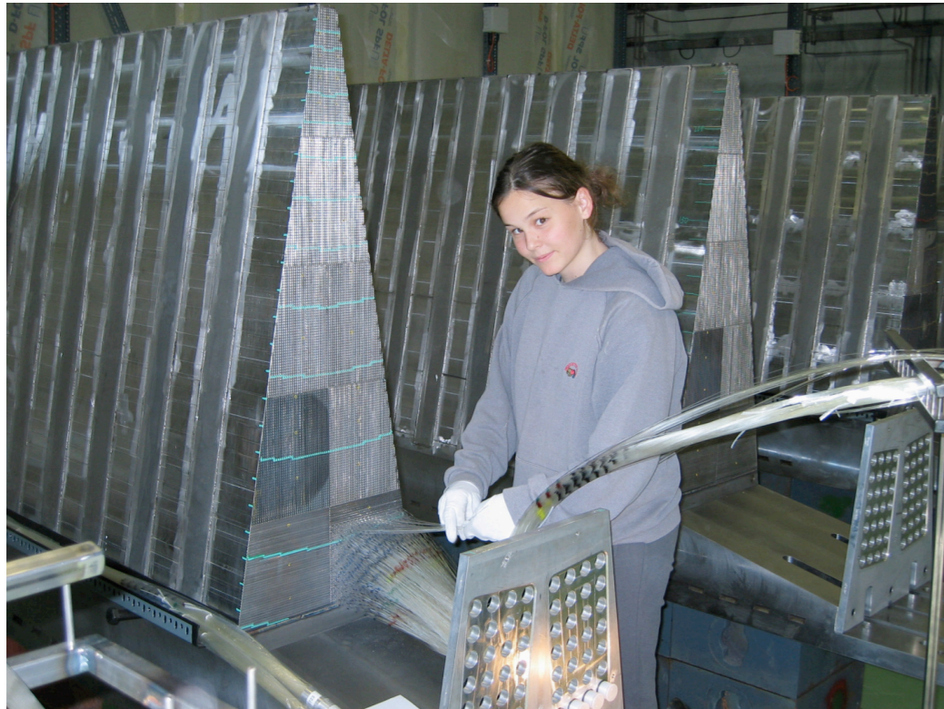
Inserting HF quartz fibres
