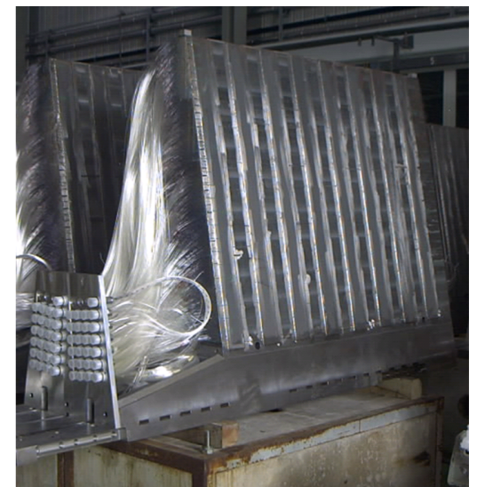
Forward (HF) Steel absorber , in 20 deg wedges Quartz fibre active element (~1000km) coverage: 3 < |\eta| < 5.0
