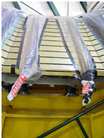
Barrel (HB) 36 brass/scintillator wedges 17 longitudinal layers 5cm brass + 3.7mm scint coverage: |\eta| < 1.3
