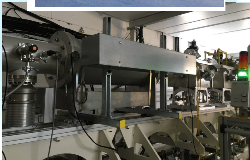
Shorter ISIS Ionisation chamber (1m long) on FETS.
