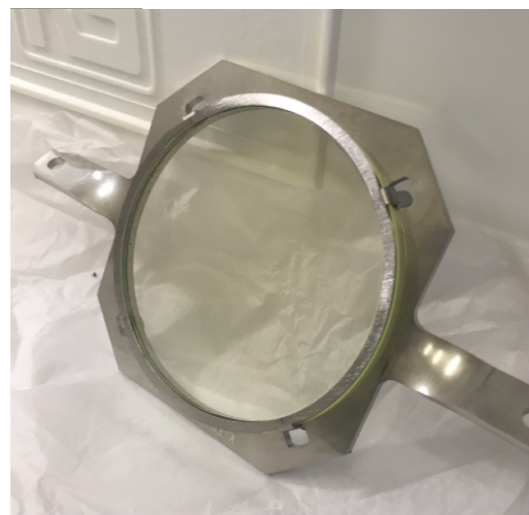
Scintillation plates for profile/position monitor
