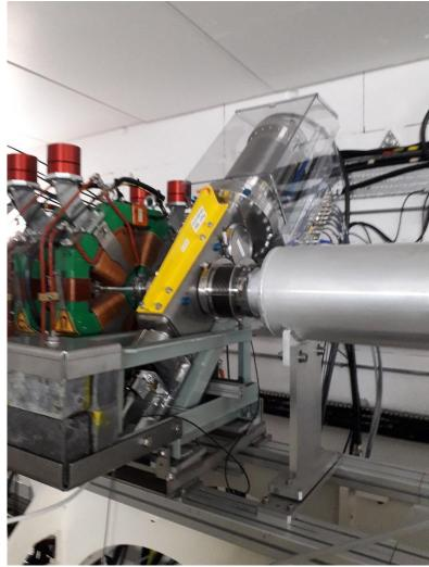
Profile monitor using carbon nanotube wires
