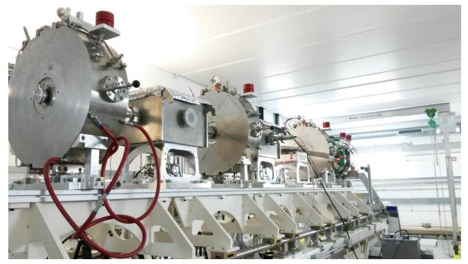
Cavities and amplifiers fully tested without beam.
