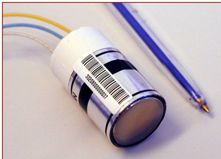
one of 14648 EE Vacuum Phototriodes (VPTs)
