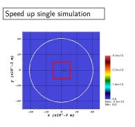
Fields are kept constant throughout the simulation (no effect of the charges induced in anode wall, ~1 kHz for rigid plasma column)
