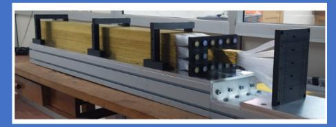
2021 test beam: EM performance test of capillary tube mechanical structure
