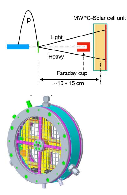
MWPC coupled to solar-cell array to study transfer-induced fission
