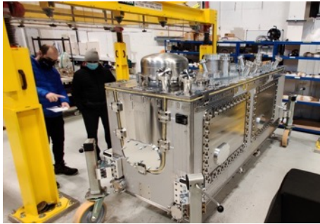
HL-LHC cryomodule at Daresbury
