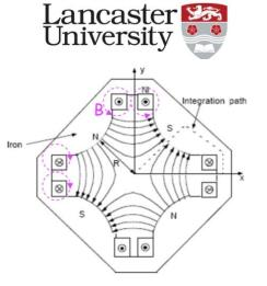
Example 1: trajectory through a quadrupole
