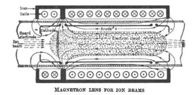
The focal length of a Gabor lens of length l is given in terms of the electron number density by:
