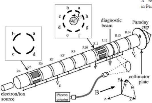
FIG. 1. Schematic of the IV Penning–Malmberg trap used for electron and ion plasma experiments. Electrons are typically confined in the region S5  $\rightarrow$  S11; Mg<sup>+</sup> ions (shown) are typically confined in the region S11 $\rightarrow$ R13. A laser diagnostic is used for ion plasmas; a collimator plate and Faraday cup diagnostic is used for electron plasmas. Azimuthally-dependent modes are driven and detected with sectored rings (S5 and S11).
