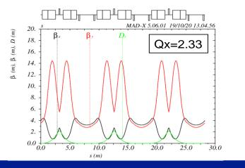
AG-CCT magnets allow periodic focusing while bending, reducing beta function (and beam size)
