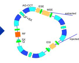
Developed within HITRI*plus* (E. Benedetto) Evolved to triangular, with 3.5 T 60<sup>o</sup> magnets and a SC quadrupole in between. No-dispersion in straight sections (inj, extr, RF)
