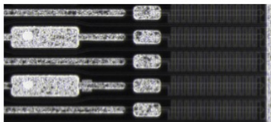
Silicon strip sensors for LHC
