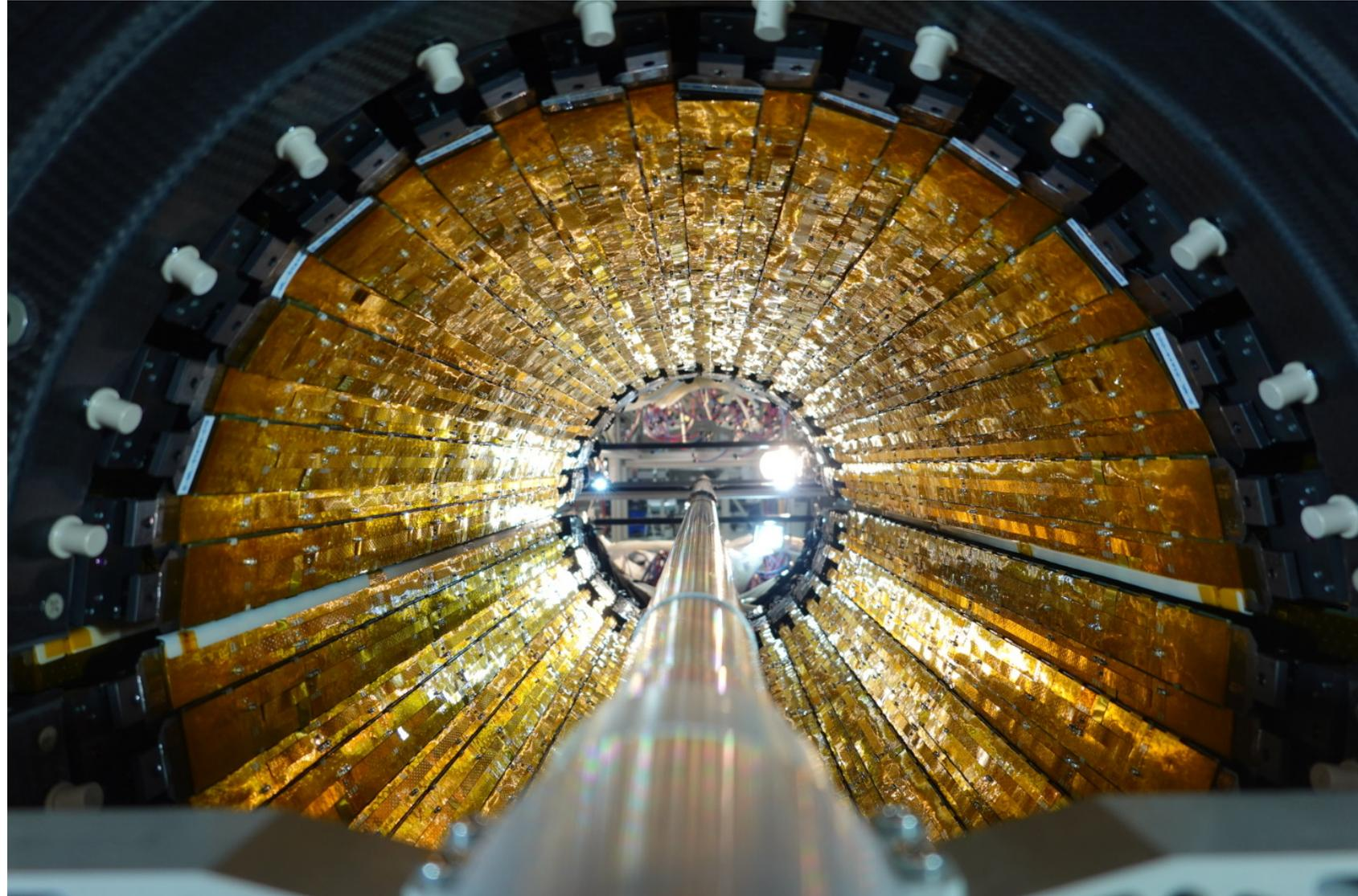
ALICE ITS2 Outer Barrel during insertion tests
