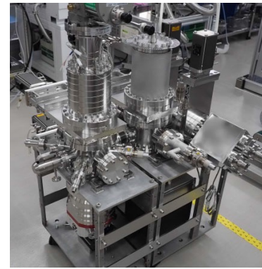
Differential pumping system (DP)
