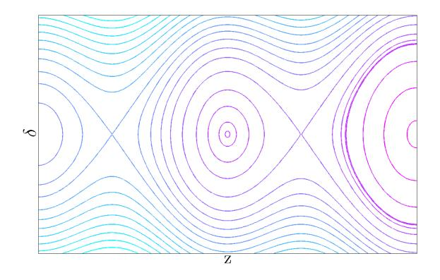
Particles follow contours in phase space of fixed value for the Hamiltonian *H*. Note that there are bounded regions where the contours form closed loops: particles in these regions perform stable oscillations. The line forming the boundary of each stable region is called a *separatrix*.
