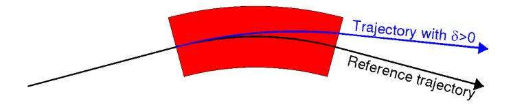
A particle with positive energy deviation ( $\delta > 0$ ) follows a *longer* trajectory in the dipole than a particle on the reference trajectory. If the particles enter with the same z, and the energy is sufficiently large (both particles travel close to the speed of light), the higher energy particle falls behind the particle with the reference energy.
