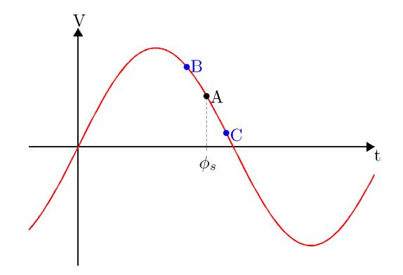
Particle *B* arrives at the RF cavity "early", and receives extra energy in addition to that lost through synchrotron radiation. If the ring is above transition, the extra energy will tend to "slow down" particle *B*. The effect is analogous to a restoring force, acting in the direction of the synchronous phase  $\phi_s$ .
