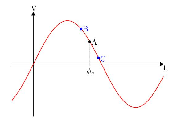
Particle A arrives at the RF cavity at the "correct" time to restore the energy lost through synchrotron radiation. The overall change in energy of particle A over one turn of the ring is zero.
