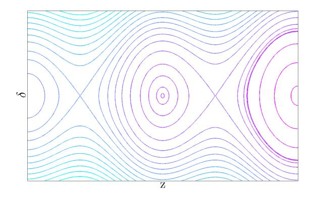
There is a maximum value for the energy deviation  $\delta$  for any particle within an RF bucket: this value is known as the *RF* bucket height,  $\delta_{max}$ . It can be shown that:
