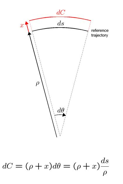
Now, consider the case that the offset x arises purely from *dispersion*, i.e. the transverse action is zero and x is a function only of the energy deviation  $\delta$ . In this case, we can write:
