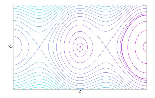
A region within a separatrix, where the particles perform stable oscillations, is known as an *RF bucket*.
