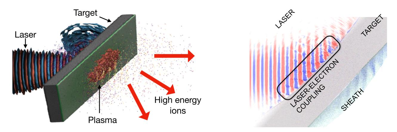
Well understood technique: target normal sheath acceleration (TNSA)
