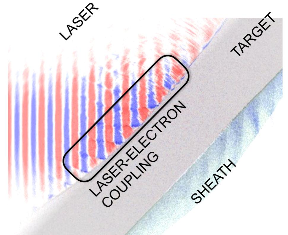
Well understood technique: **target normal sheath acceleration (TNSA)**
