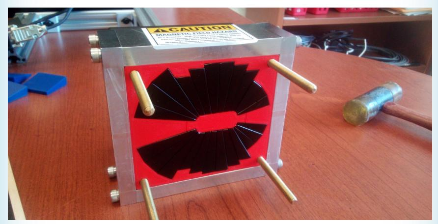
Outer <sup>1</sup>/<sub>2</sub>" thick aluminium frame for strength
