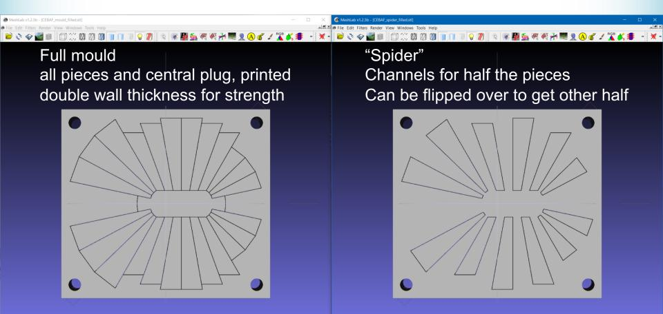
Corner holes for 1/4"-20 threaded rods throughout, provide loose alignment, constraint
