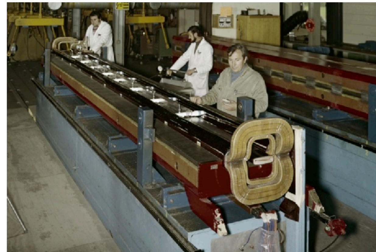
Fig. 3: The B_{\max} = 2.05 T SPS dipole magnet: left, the cross-section, right, a photograph taken during assembly in the early 1970s.
