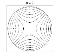
Field focusses in one transverse direction, defocusses in the other
