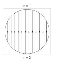
Geometric focussing effect perpendicular to dipole field (aka weak focussing)
