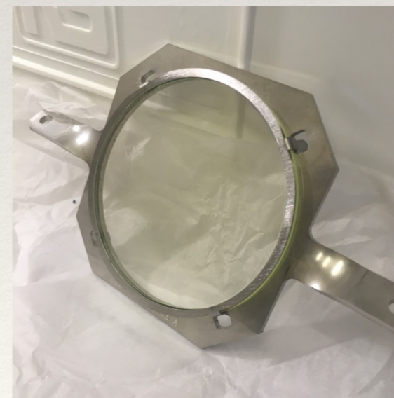
Fig.2 Screen mount folder to be installed on WSM head.
