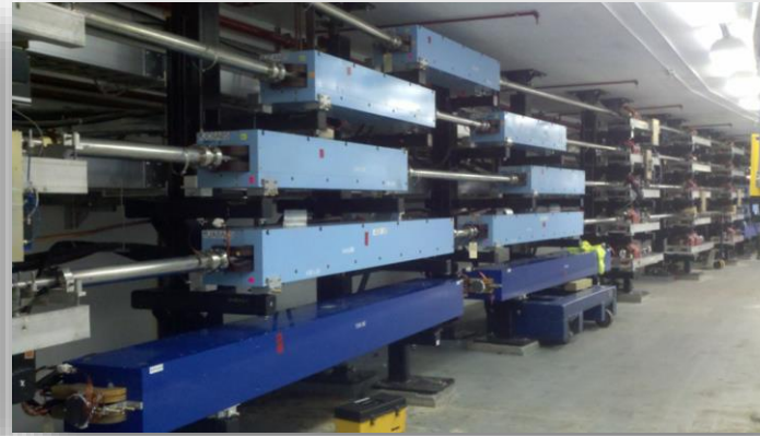
~500 Large Dipoles powered by >40 HVPS
