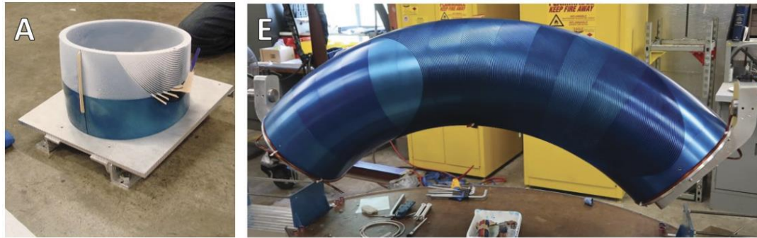
▲ LBNL 90° AG-CCT prototype using laminated mandrel (anodized aluminum)
