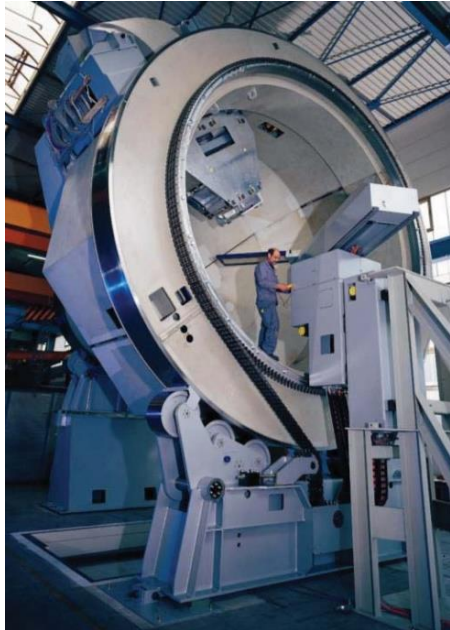
Normal-conducting gantry, >200 tons (PSI Gantry 3)
