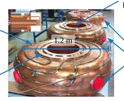
Internal surfaces treated to suppress breakdown
