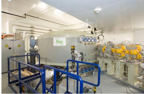
IBA normal-conducting, 230 MeV
