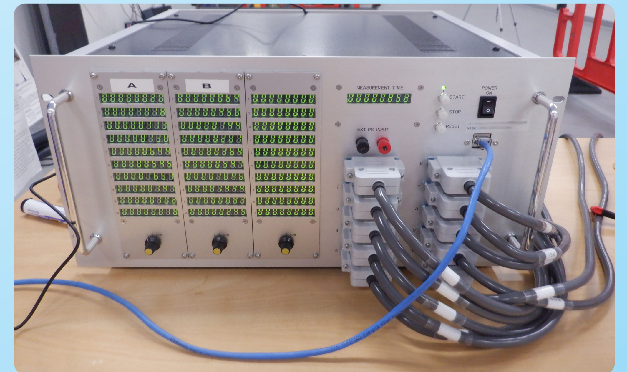
Figure 3 (right): Main control unit. Readouts A and B show PMT singles rates, final readout gives coincidence rates.
