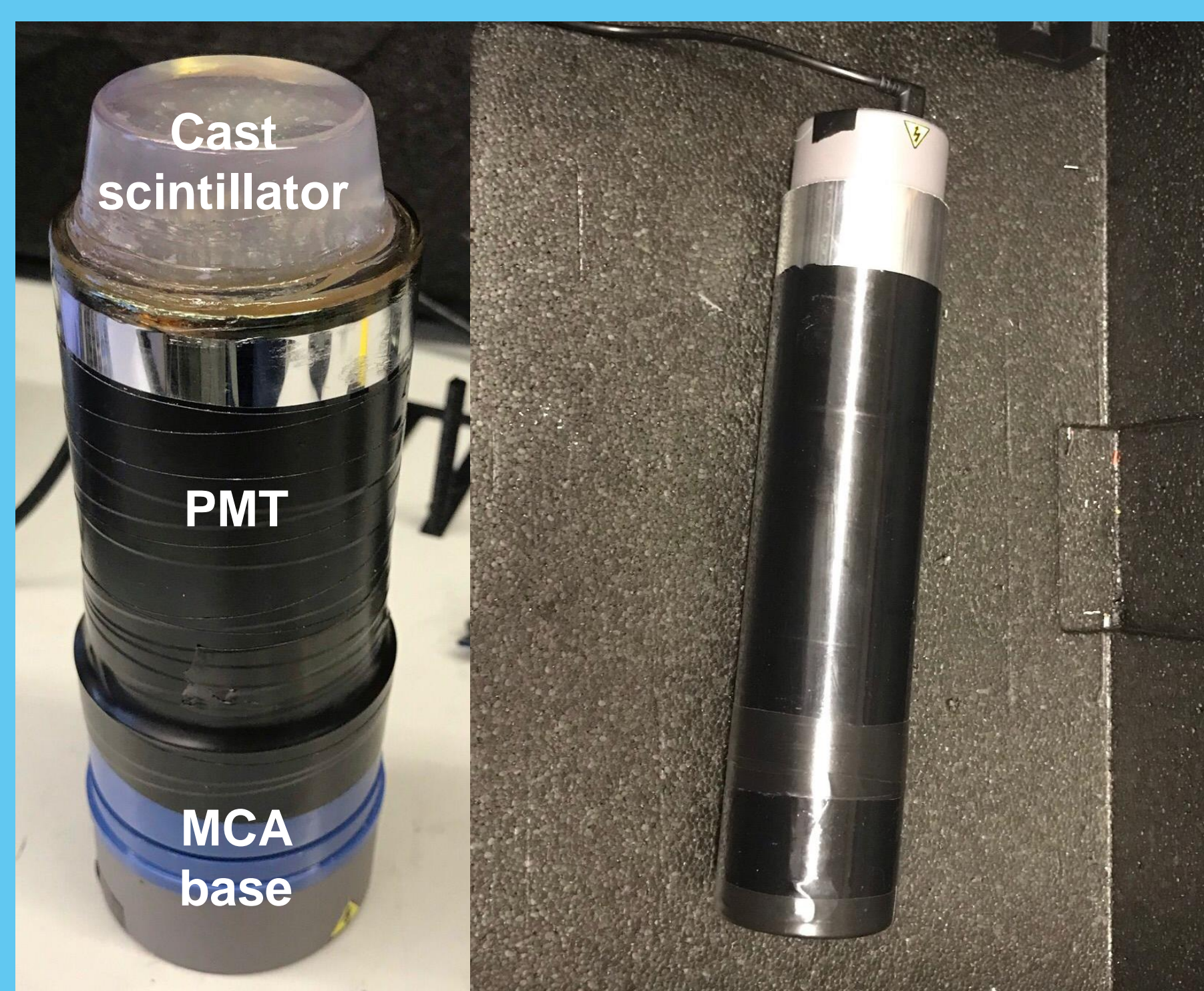
Figure 4: Sample coupled directly to PMT face (left) placed in light tight assembly (right)
