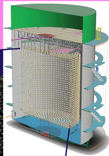
Figure 1: Cutaway of the cylindrical tank used.
