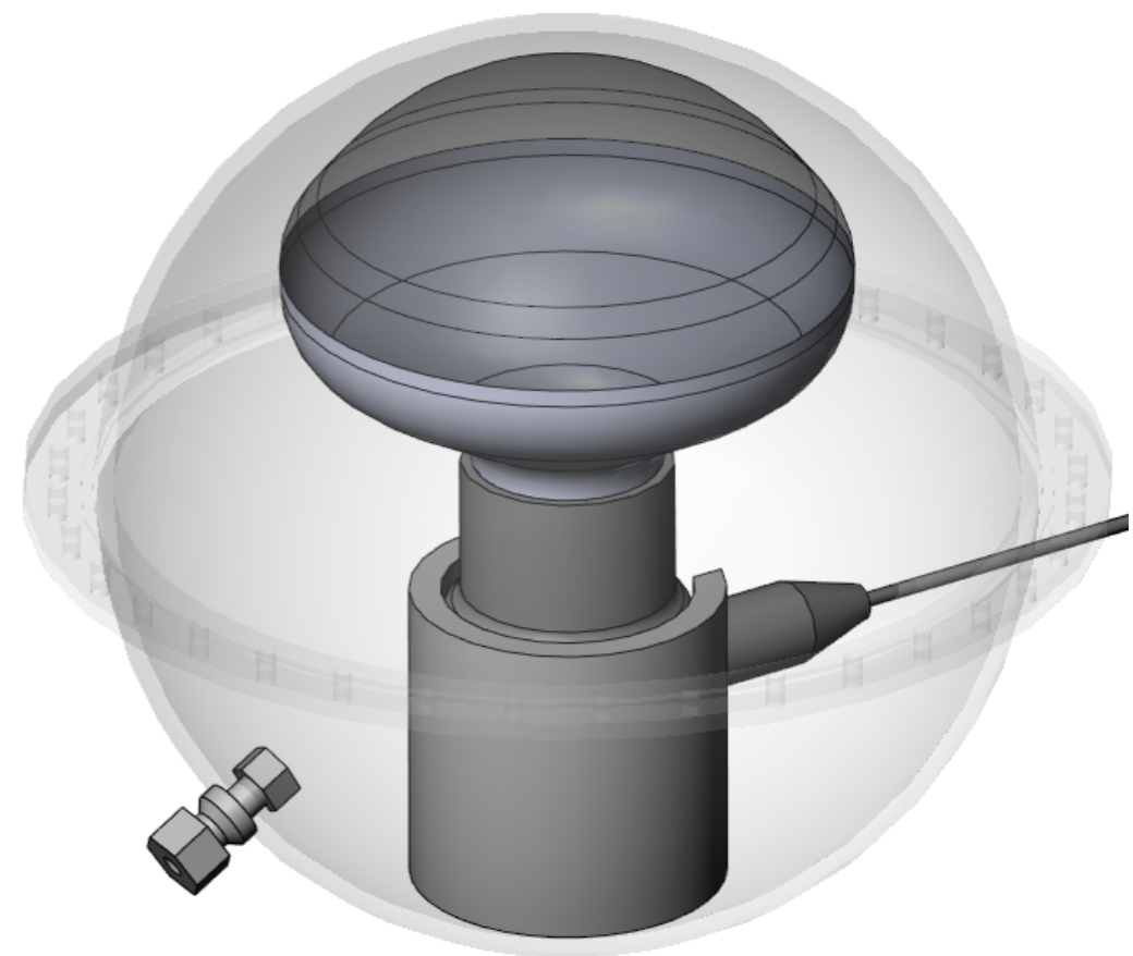
UVT acrylic PMT module. Image from Edinburgh group. Modules developed by Edinburgh and ICL Tech.
