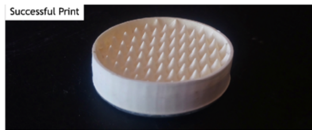
3D Printing Neutron Detectors using Scintillating BN/ZnS Resin
