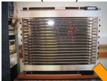
Spark Chamber S.Fukui, S.Miyamoto (~1958)
