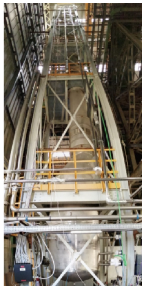
ARIA project (Darkside Collab.), production of depleted argon, below the UAr levels
