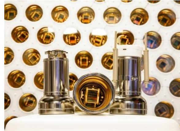
LZ Hamamatsu R11410 0.007 \gamma /s/PMT Akerib 2020
