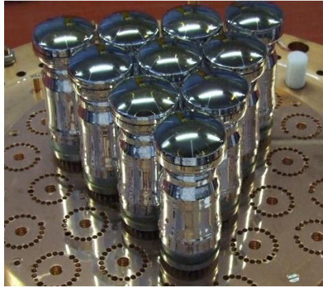
ZEPLIN-III SSR / ETEL D766Q 0.044 \gamma /s/PMT Araujo 2012
