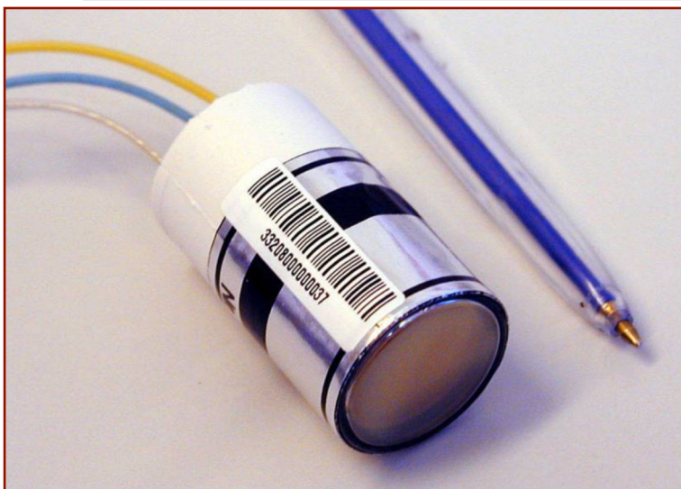
one of 14648 EE Vacuum Phototriodes (VPTs)
