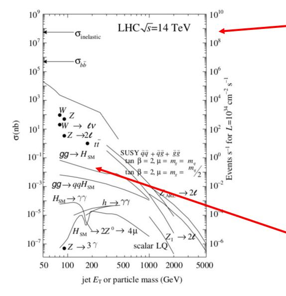
Inelastic cross-section -> GHz of events (40MHz bunch crossing x ~40 p-p interactions per crossing)
