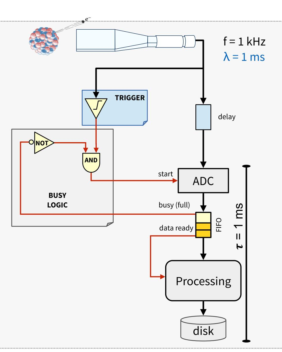
The FIFO decouples the low latency front-end from the data processing
