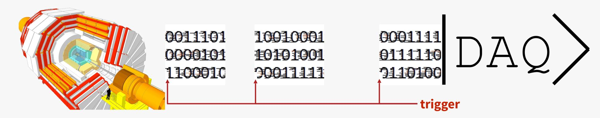
Streaming: detector pushes all its data and the downstream DAQ must keep the pace
