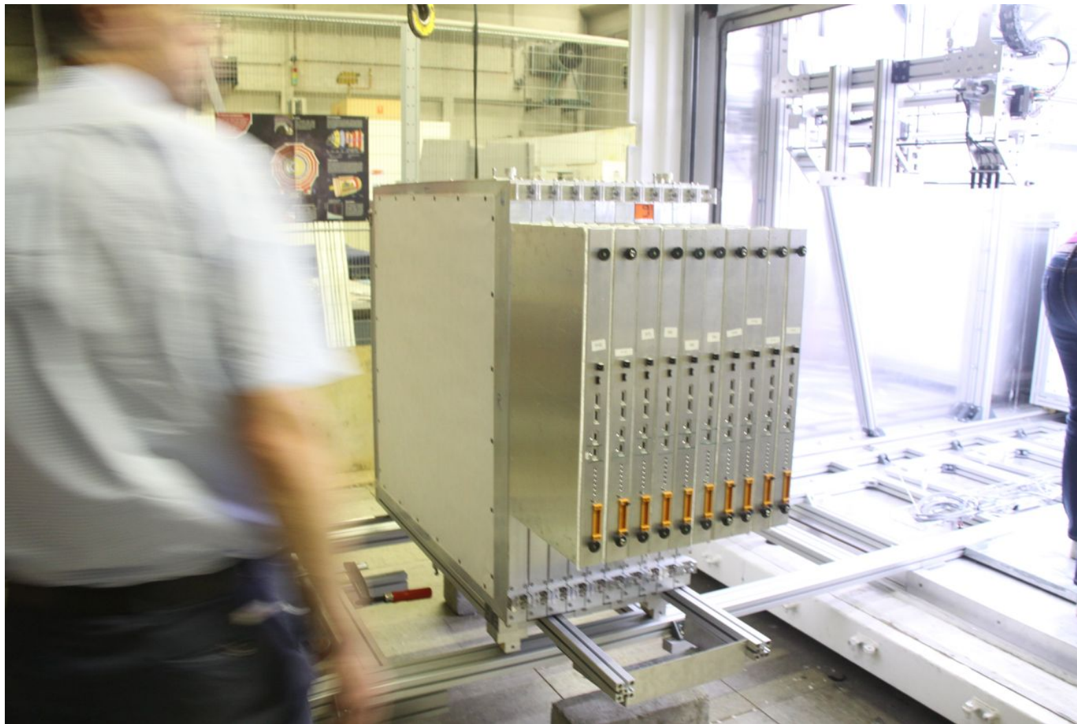
Fig: Example detector module of ten planes.
