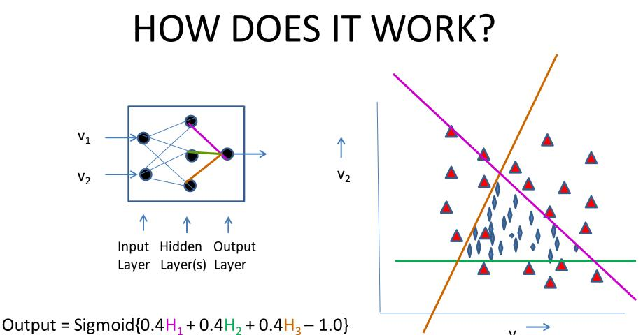
Output is 'On' only if  $H_1 H_2 H_3$  all are 'On'
